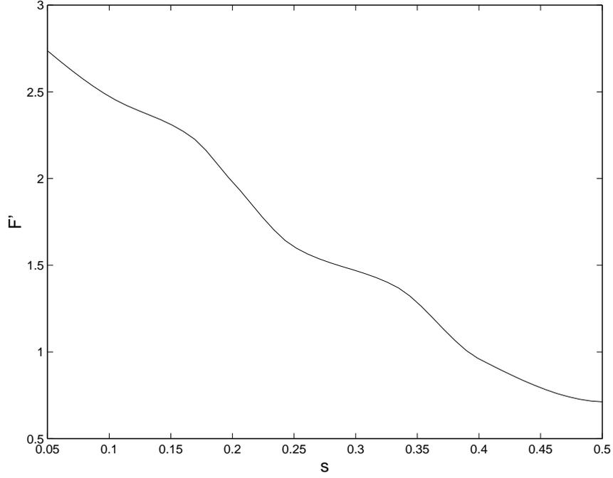
Fig. 5.3 – Dependence of the dimensionless drag force  $F'$  on the dimensionless distance  $s$  for  $h/a = 10$ .
