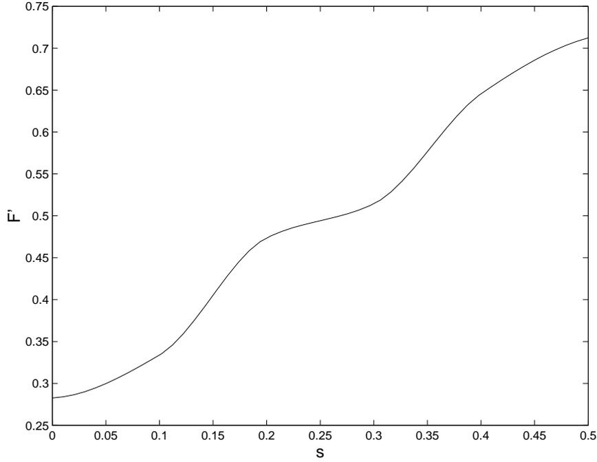
Fig. 5.4 – Dependence of the dimensionless drag force  $F'$  on the dimensionless distance  $s$  for  $c = 10$ .
