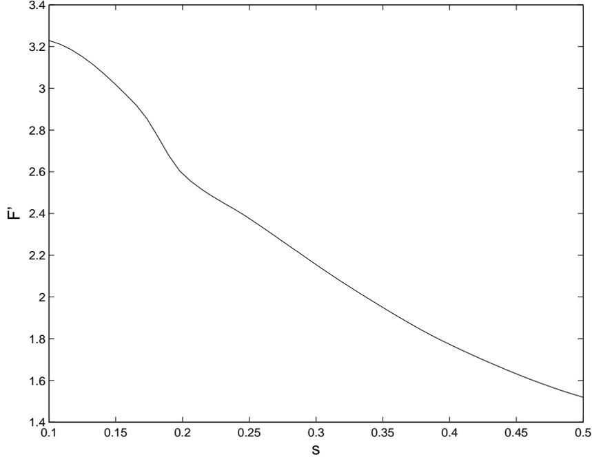
Fig. 5.2 – Dependence of the dimensionless drag force  $F'$  on the dimensionless distance  $s$  for  $h/a = 5$ .
