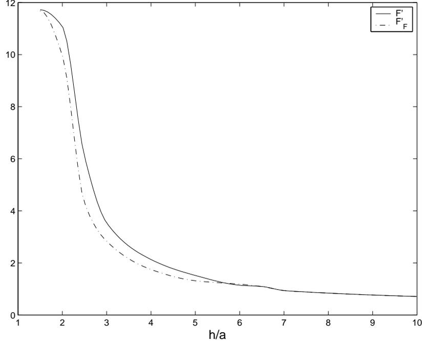
Fig. 5.1 – Dependence of  $F'$  and respectively  $F'_F$  on the ratio  $h/a$ : parallel motion.
